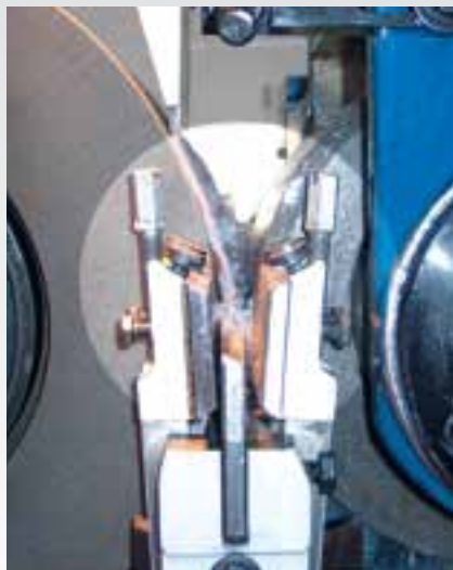
Example: work rest blade in use during grinding process
